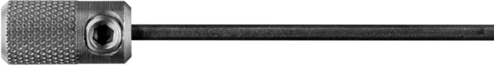
(a) **Loosen the set screw** in the handle which also serves as a protective cover for the **delicate, .028" dia. twist drill**. Slowly slide the handle to the far end of the shaft and lock it in place **using care to not bend or break the drill bit.** **Do not over-tighten the set screw** as this can damage the shaft.
